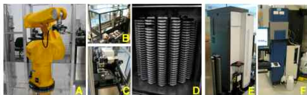
Fig. 1. The Scripps Research uHTS platform. A, An industrial anthropomorphic robotic arm moves assay and compound microtiter plates. B, A pin tool is used to transfer test compounds rapidly from compound plates to assay plates. C, Liquid handlers capable of dispensing up to 32 different reagents and of washing plates are integrated into the platform. D, Incubators, each capable of holding approximately 700,000 samples in 1536-well format, are used to store microtiter plates at a variety of temperatures and gas concentrations. E, A multimode plate reader measures absorbance, luminescence, fluorescence, or fluorescence resonance energy transfer (with time resolution) from microtiter plates. F, A kinetic imaging plate reader allows measurement of second-messenger or ion channel activity in live cells. Not shown is a compound management robot capable of storing and retrieving desirable compounds from the Scripps Research screening file.
