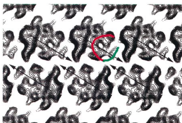
Figure 3. Contour plot of an electron density projection map of the p1 (acetate) crystals (preserved in amorphous ice) formed by wild-type RNA polymerase II. The unit cell parameters for these (acetate) crystals are a = 125.4 \text{ \AA} , b = 227.5 \text{ \AA} , \beta = 106.1^\circ . As was observed for crystals of the \Delta 4/7 enzyme formed under the same buffer conditions, the crystal is composed of antiparallel rows of monomers, all interacting with the charged lipid layer through the same face of the molecule. However, comparison with the projection map shown in Figure 1 indicates that the wild-type enzyme is in the closed conformation, and that there has been a packing rearrangement to accommodate the extra density present in the plane of the crystal. As indicated by the arrows, all the monomers have rotated \sim 30^\circ clockwise with respect to the orientation observed when the enzyme is in the open conformation, and the protein density immediately behind the arrowheads (under the green portion of the arch that traces the position of the domains that define the DNA-binding cleft) blocks access to the DNA-binding channel.
